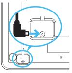
Run the power cable through the canal on the bottom of the XL Pro.
